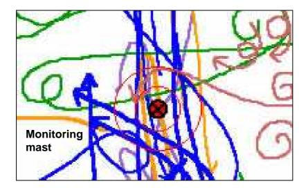
Figure 5: Flights in the proximity of the guyed monitoring mast recorded after 68.42 hours of observation (red circles indicate 100m and 200m proximity zones around the mast).
