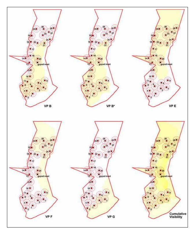
Figure 3: the 20m A.G.L. visible areas in the wind farm envelope are shown shaded in yellow for each vantage point and in combination (increased cumulative visibility is indicated by darker shading).
